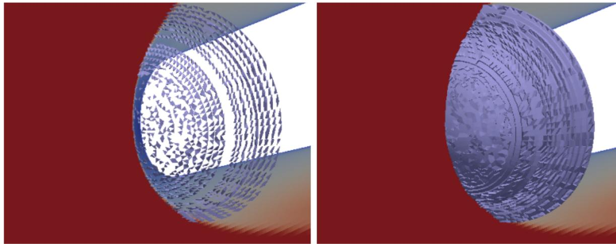
Shock elements for the HiFiRE-I case on a medium mesh: (left) before processing and (right) after processing
