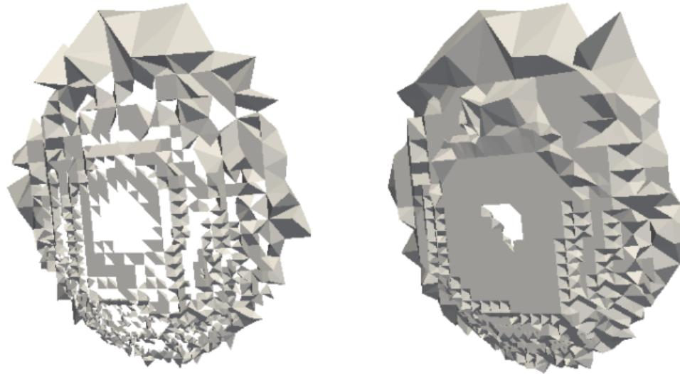
Shock elements for the CEV case on a coarse mesh: (left) before processing and (right) after processing
