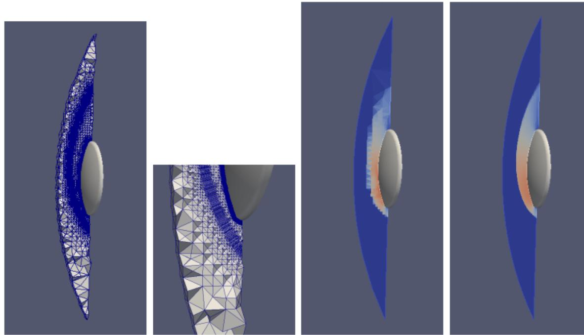
Shock-fitted mesh: (left) full and zoomed views, and (right) solution on coarse and fitted meshes
