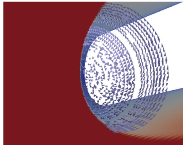
HIFiRE-I case: near-nose shock elements on a medium mesh
